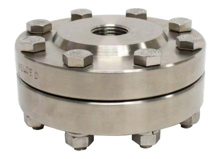
The Model 14040 Welded Diaphragm Seal is a welded diaphragm-to-upper design allowing the upper housing to be removed with the instrument in place without losing fill. Available in threaded connections for pressures from vacuum to 2,500 psi. Fill/bleed port screw in the upper is standard and an optional flush connection is available.
