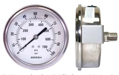
Marsh Instruments Severe Service Liquid Filled Gauges are designed to perform in rugged and harsh environmental conditions, especially where pulsation or vibration is a problem. Liquid Filled Gauges offer a significant cushioning and dampening effect, reducing pointer flutter and lubricating the internals.
