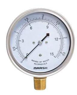
Low Pressure Gauges from Marsh Instruments incorporate a diaphragm element allowing for accurate low-pressure readings in support of a variety of applications, with ASME Grade A 2/1/2% accuracy for ranges above 30" of water. Available ranges include vacuum and pressure in inches of water, ounces per square inch, kilopascals, and millimeters of mercury.
