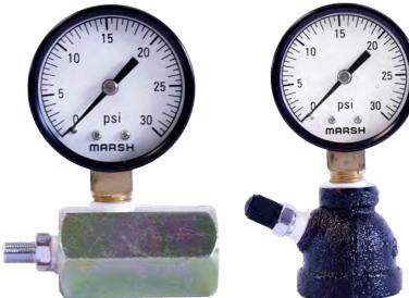
Used to pressure test all new gas installations for leaks and passing inspection codes. After installing the Marsh Instruments Gas Test Gauge, the system is pressurized with air. Any leakage will be indicated by a pressure drop in the gauge.
