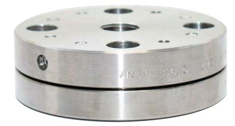
The Model 140FL Welded Diaphragm Seal is a welded diaphragm-to-upper design allowing the upper housing to be removed with the instrument in place without losing fill. Available in threaded connections for pressures from vacuum to 2,500 psi. Fill/ bleed port screw in the upper is standard and a flush ring option is available.
