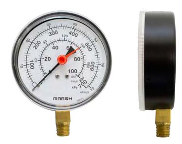
Marsh Instruments Heating System Gauges are available in 3 1/2" and 4 1/2" dial sizes. An adjustable red altitude pointer is standard on feet of water gauges. This feature allows the user to indicate the head of water to be maintained in the system Marsh Instruments Heating System Gauges provide accurate psi and feet of water measurements in elevated tanks, reservoirs, standpipes, and similar applications where reliability and dependability are crucial in heating system equipment.
