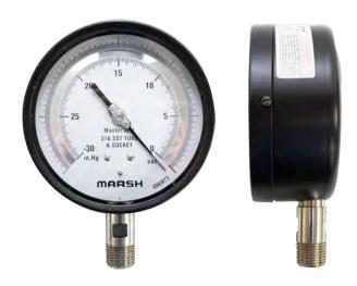
The Marsh Instruments Test Gauge is designed with a black painted steel housing and 316 stainless steel tube and socket to meet the demanding service needs of various test gauge applications. Accuracy is 0.5% of full span. A highly polished integral mirror is positioned between the two graduation arcs on the dial face. The knife-edge pointer is reflective so that, when the pointer and it's reflection are in alignment, parallax is virtually eliminated and a true dial reading is assured.
