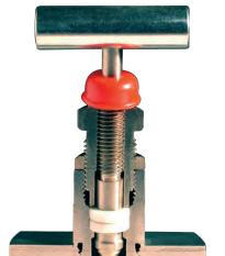
For applications where bubble-tight shutoff of liquids or gases are required. Pressure rating to 6,000 psi (42,000 kPa). These valves are designed with a replaceable Delrin soft seat.
