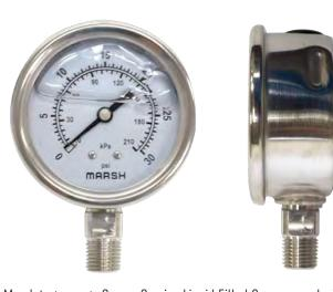
Marsh Instruments Severe Service Liquid Filled Gauges are designed to perform in rugged and harsh environmental conditions, especially where pulsation or vibration is a problem. Liquid Filled Gauges offer a significant cushioning and dampening effect, reducing pointer flutter and lubricating the internals.
