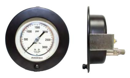
The Marsh Instruments Test Gauge is designed with a black painted steel housing and 316 stainless steel tube and socket to meet the demanding service needs of various test gauge applications. Accuracy is 0.5% of full span. A highly polished integral mirror is positioned between the two graduation arcs on the dial face. The knife-edge pointer is reflective so that, when the pointer and its reflection are in alignment, parallax is virtually eliminated and a true dial reading is assured.
