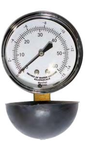
The Marsh Instruments Vacuum Cleaner Test Gauge is designed to test the amount of vacuum generated by a vacuum cleaner to ensure proper operation and to check for leaks or other problems. The Vacuum Cleaner test gauge features a reliable Marsh Instruments Low Pressure Diaphragm Gauge available in several ranges, as well as a rubber plug/fitting designed to fit various different vacuum cleaner hoses and connections.
