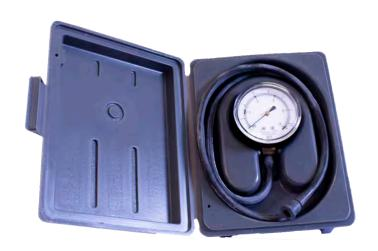
The Marsh Instruments Gas Pressure Test kit is designed to test the system pressure of your natural gas or LP system. It can be used to check for leaks as well as accurately set manifold pressure. The kit includes an easy-to-read Marsh Instruments low pressure diaphragm gauge, 30" long hose and fitting all contained in a durable case to help protect the instrument and allow for easy transport.
