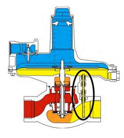
The P134 has an onboard registration tube, circled in the figure at left, allowing for the regulator to be installed without the external pressure registration necessary on the P133.
