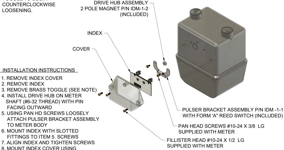
IMPORTANT!! GUIDE SWITCH WIRES AROUND INDEX TO CLEAR GEARS. CONTINUE GUIDING WIRES AND EXIT COVER THROUGH BOTTOM LUG OR HOLE ABOVE RIGHT SCREW
