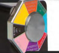
Most Manual & Hydraulic squeeze off tools feature positive locking, indexable gauge plates for easy selection of size & SDR to ensure a proper squeeze.
