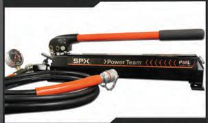
Lightweight single stage hydraulic hand pump c/w pressure gauge lock out needle valve and 15' hose. For model C165-AK1
