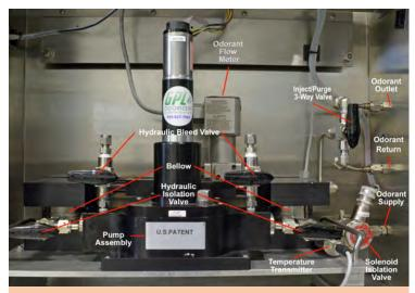
Solid-state modular design permits hot-swap capability, minimal joints, and tubing for long lasting performance.
