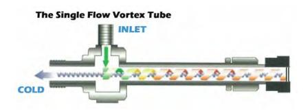
In the VPR, high pressure gas expands in the unit's tangential nozzle of a fixed size down to the delivery pressure. While in the VPR cylindrical
