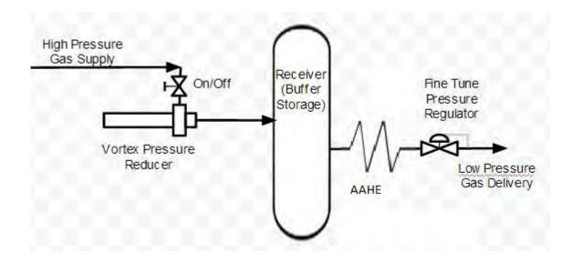
From the flow control stand point a buffer receiver (inter-stage storage) fed through the VPR's fixed, unchangeable (no moving part!) inlet nozzle *allows delivering a variable flow to the end user.*
