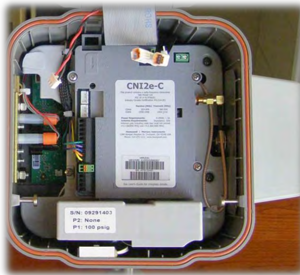
Figure 3. The EC 350's internal digital cellular radio meets the specific needs of gas applications.
