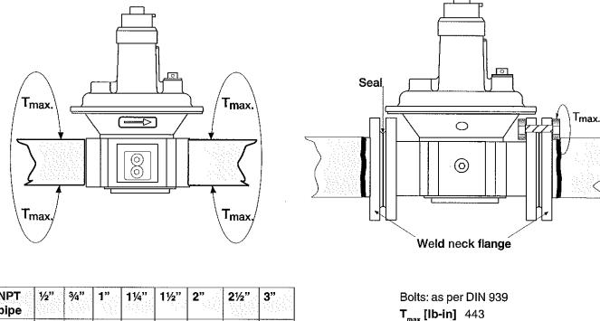
NOTE: There are no limits for required pipe lengths immediately downstream of the FRS.
