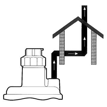
In the absence of venting codes and where venting is required, each regulator must be vented separately from all other vents.
